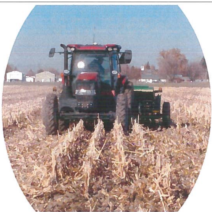
Canyon SCD No-Till Drill (2020 Great Plains) planting cover crops in standing corn residue
